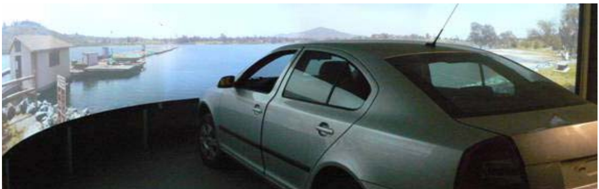
Fig. 1 Compact simulator type II with surrounding projection (not fully finished – dummy scenery)
