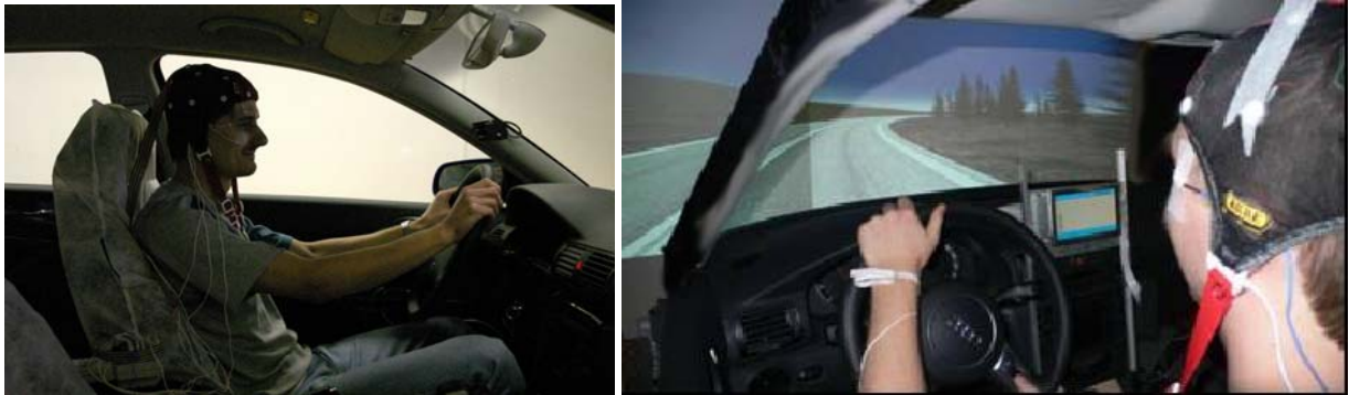
Fig. 3 The tested driver equipped with EEG cap and heart beat recording (Compact simulator type I – left, Light simulator type I – right)
